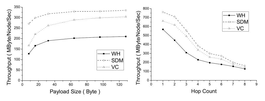
All routers approach the maximal throughput with longer payload length. FL=64 Byte shows 90% maximal throughput. Throughput decreases with the increasing hop count. SDM shows better through even in the 8-hop case
