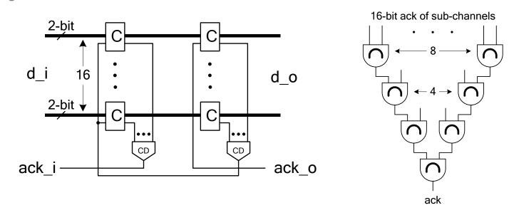
Advantages: data on all sub-channels are synchronized, ease the time division multiple access (TDMA) techniques, such as virtual channel and TDMA
