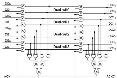
Fig. 1. A dual-rail pipelined channel
