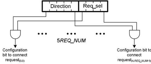
Fig. 8. The request configuration register of a request in the transmission control
