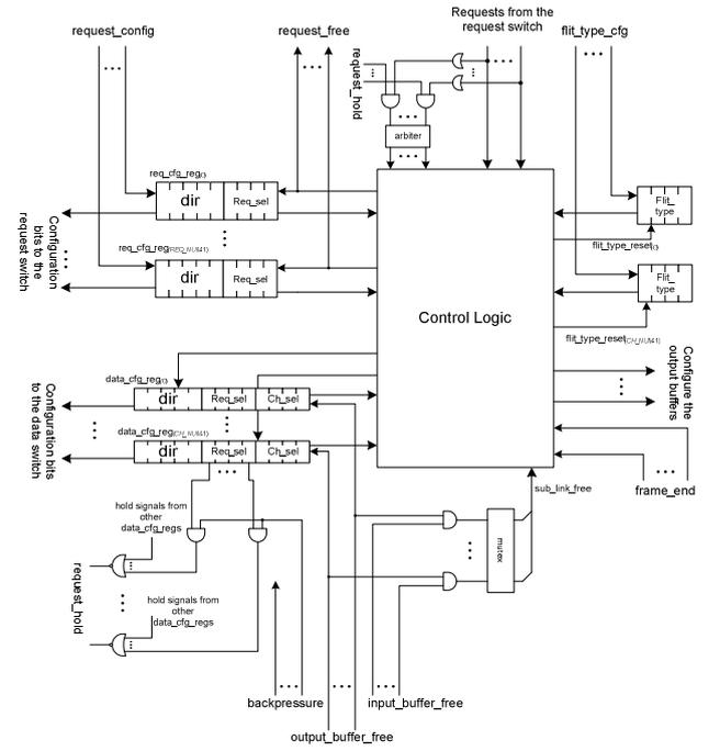
Fig. 9. The internal structure of the transmission control
